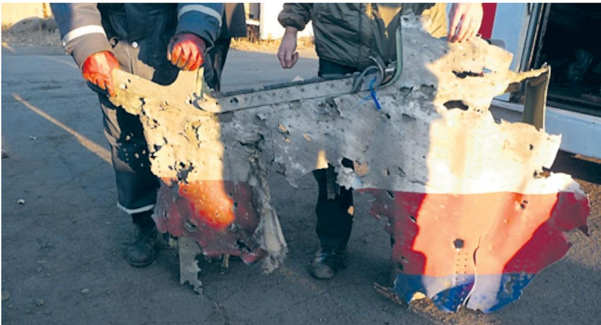
*Figure 32: Handover of the left cockpit window frame to the Dutch Safety Board by members of the SES. This is the same part as is shown in Figure 33. (Source: Dutch Safety Board)*
