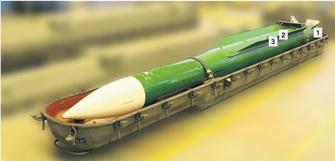
Figure 35: Image of 9M38M1 surface-to-air missile showing the approximate location of three of the parts recovered. (Source: NBAAI)
