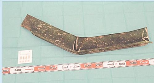
Part of stabilizing fin during identification at Gilze-Rijen Air Force Base. (Source: Dutch Safety Board/Dutch National Police)
