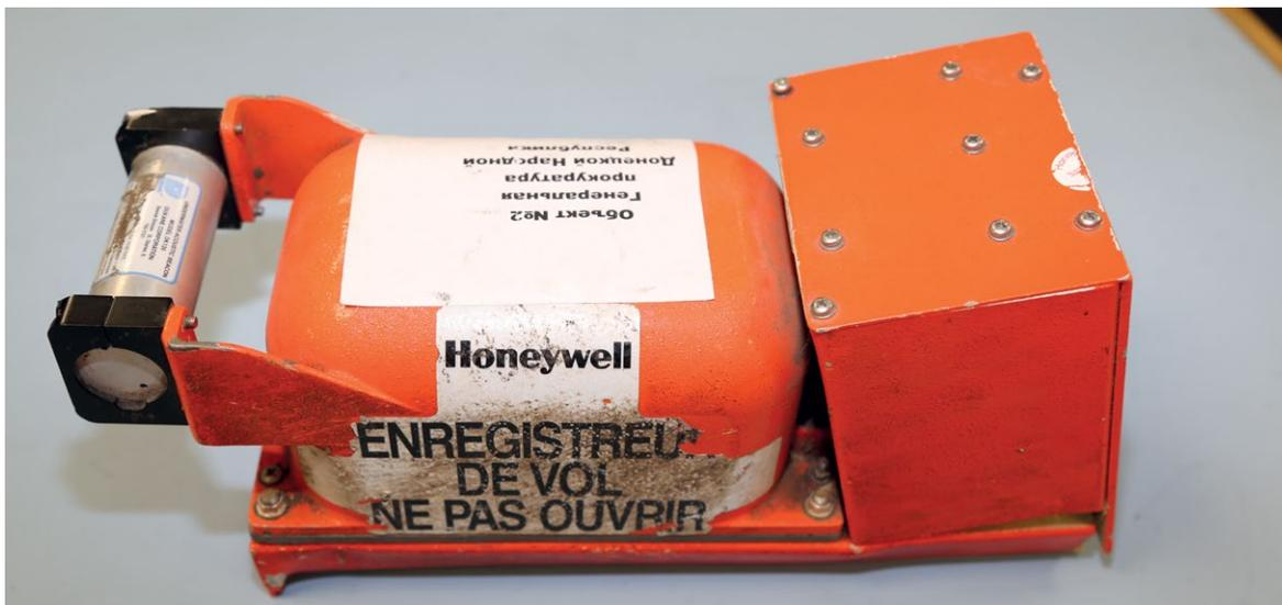
Figure 8: Cockpit Voice Recorder. (Source: Dutch Safety Board)
