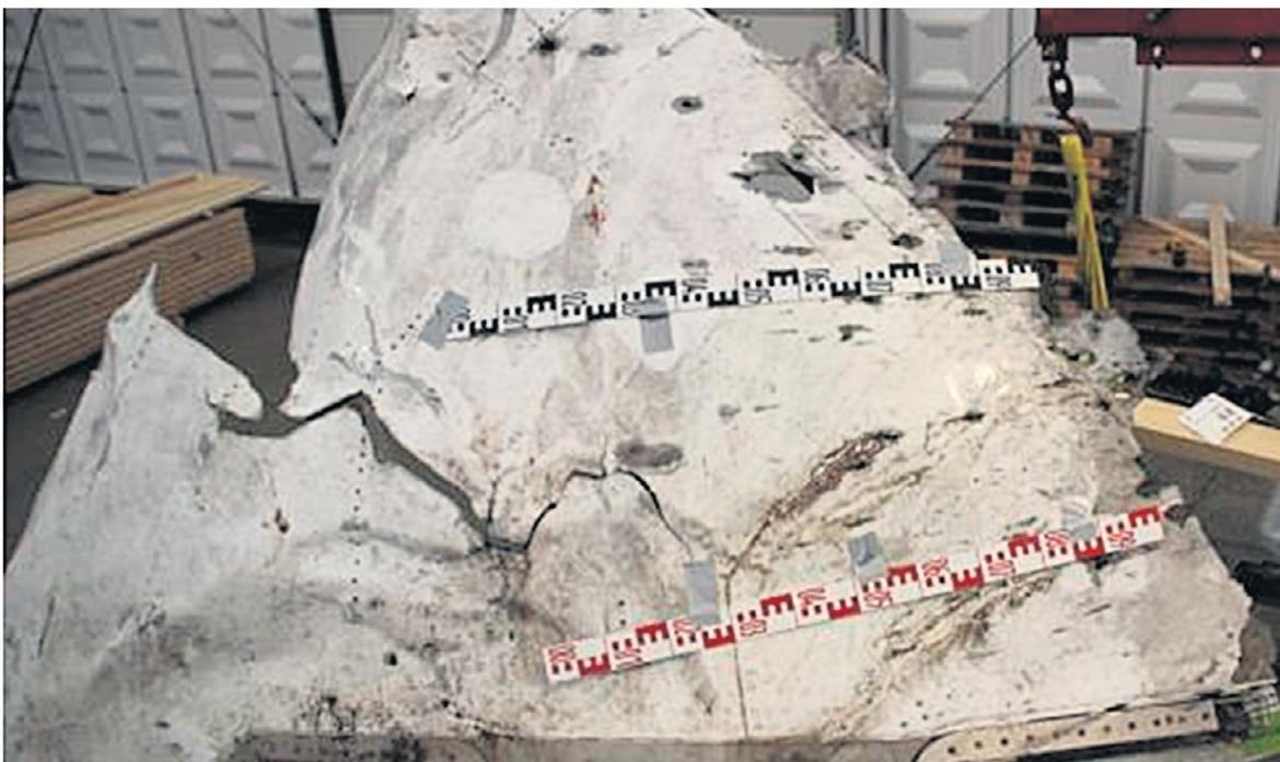
Figure 49: Grazing on cockpit roof. (Source: NLR)
