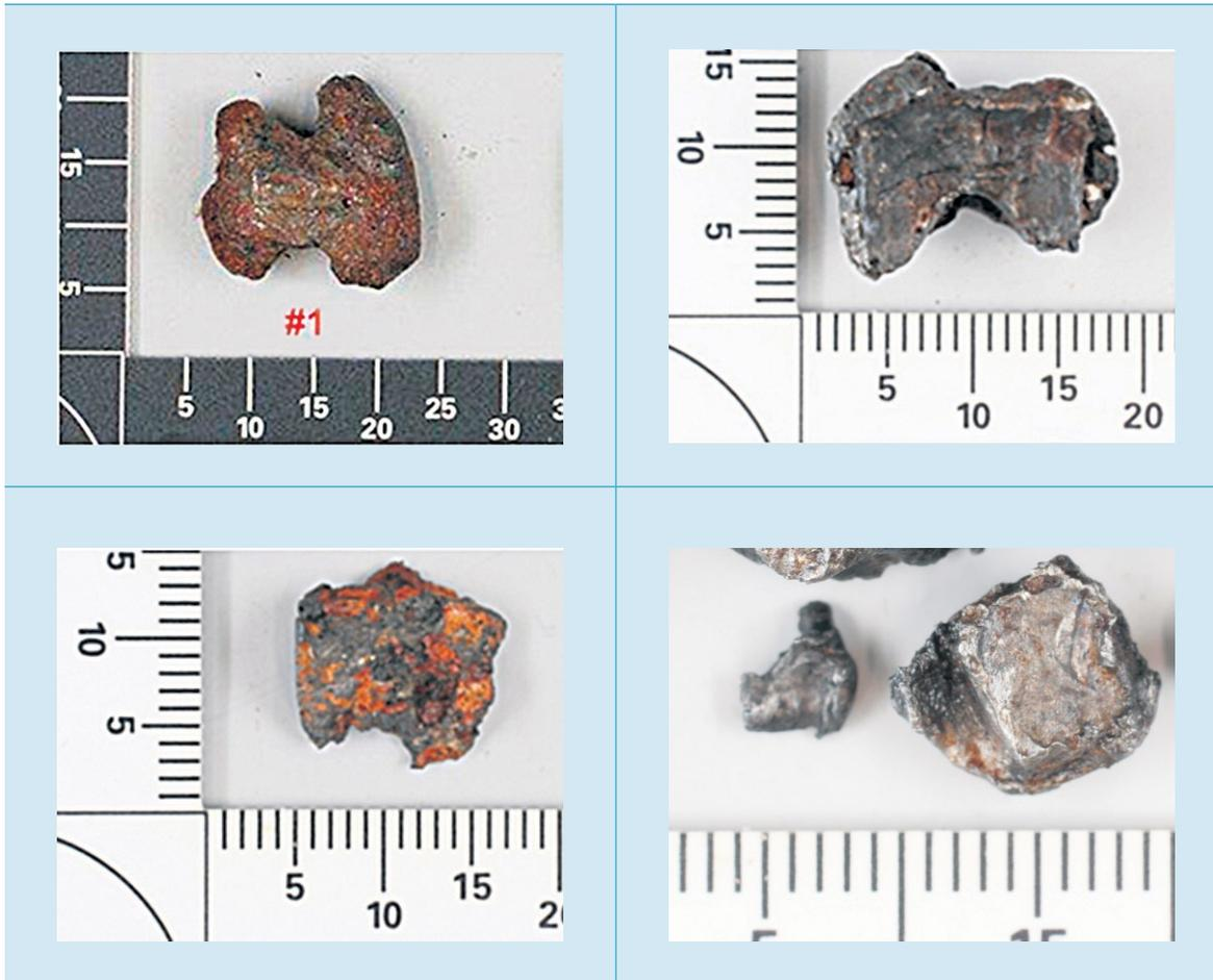
Figure 37: Four distinctly shaped fragments. Top left: cockpit. Top right: Captain's body. Bottom left: Purser's body. Bottom right: First Officer's body. (Source: NFI). Scale is in millimetres.
